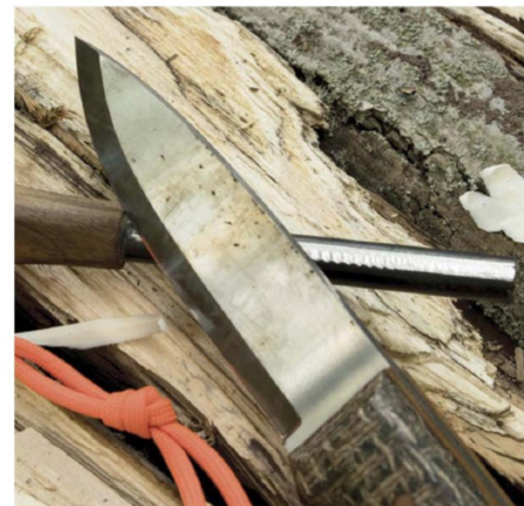
Left: The spine was completely undamaged and only had some dust from the ferro rod, which wiped off easily.
