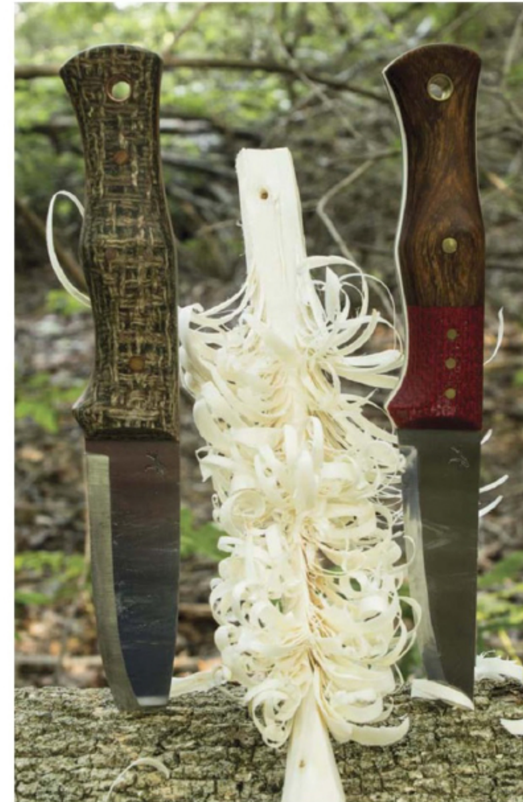
Left: The curls I got from the Camper (on the right side of the stick) were a little lighter than those from the Nomad (on the left side of the stick) due to its keener edge.
