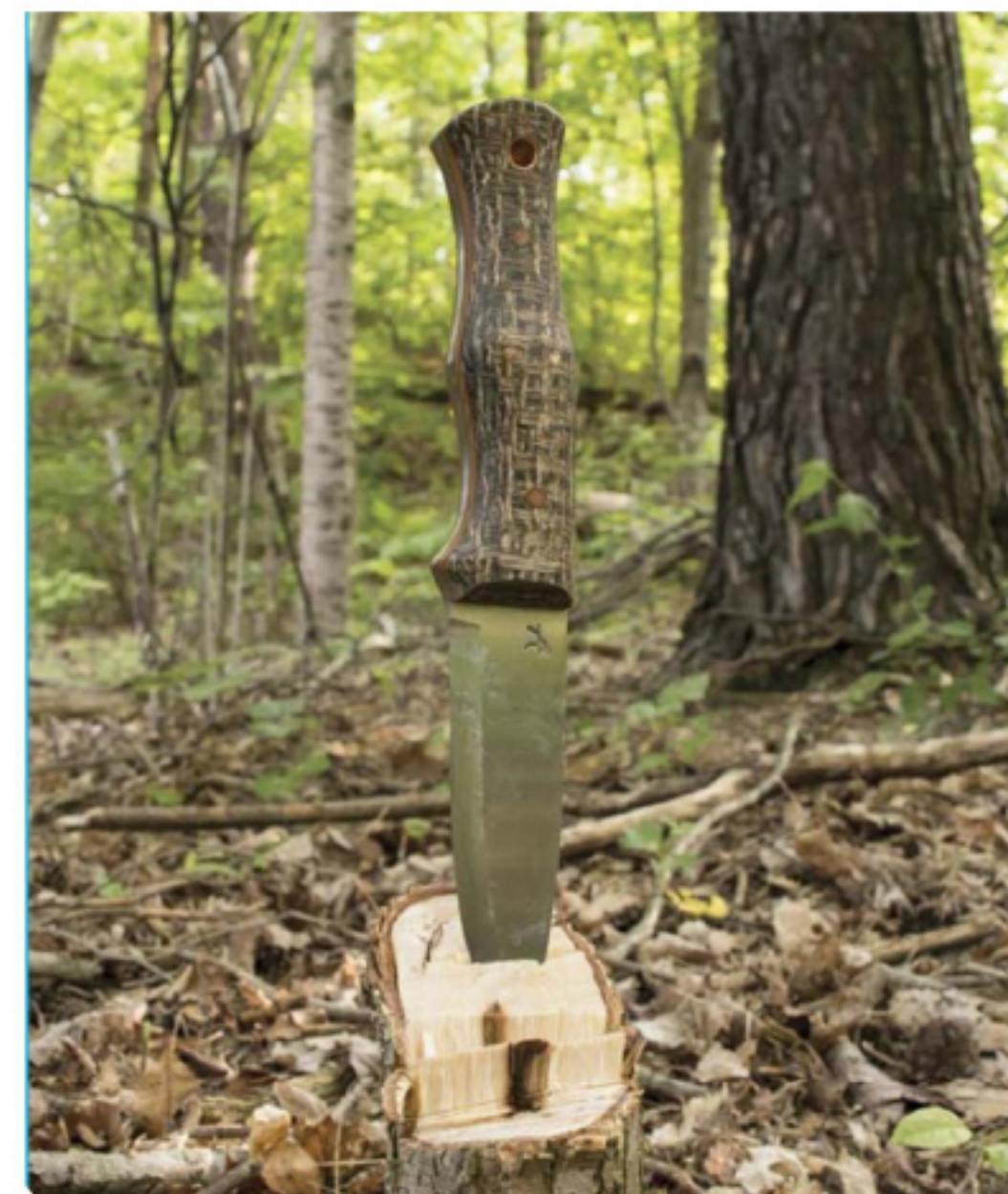
Left: After notching the front of the round and finishing with a back cut, the 3-inch round fell easily.
