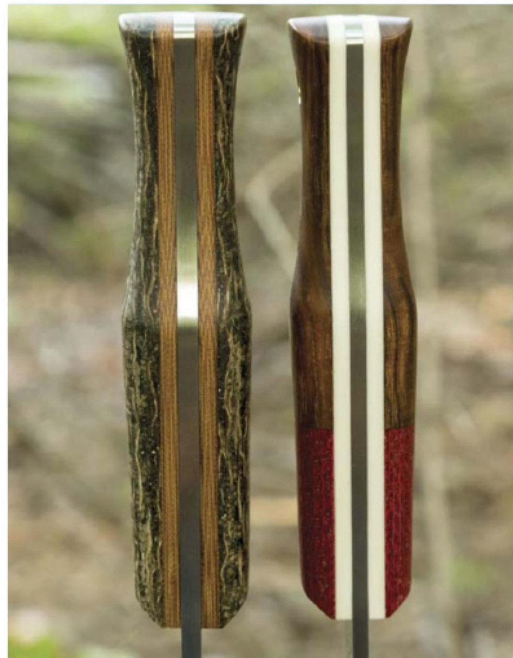
Right: The handle contouring on both knives made them really comfortable to use. You can see from this photo that the stock used on the Camper (right) is much thinner than that of the Nomad (left).
