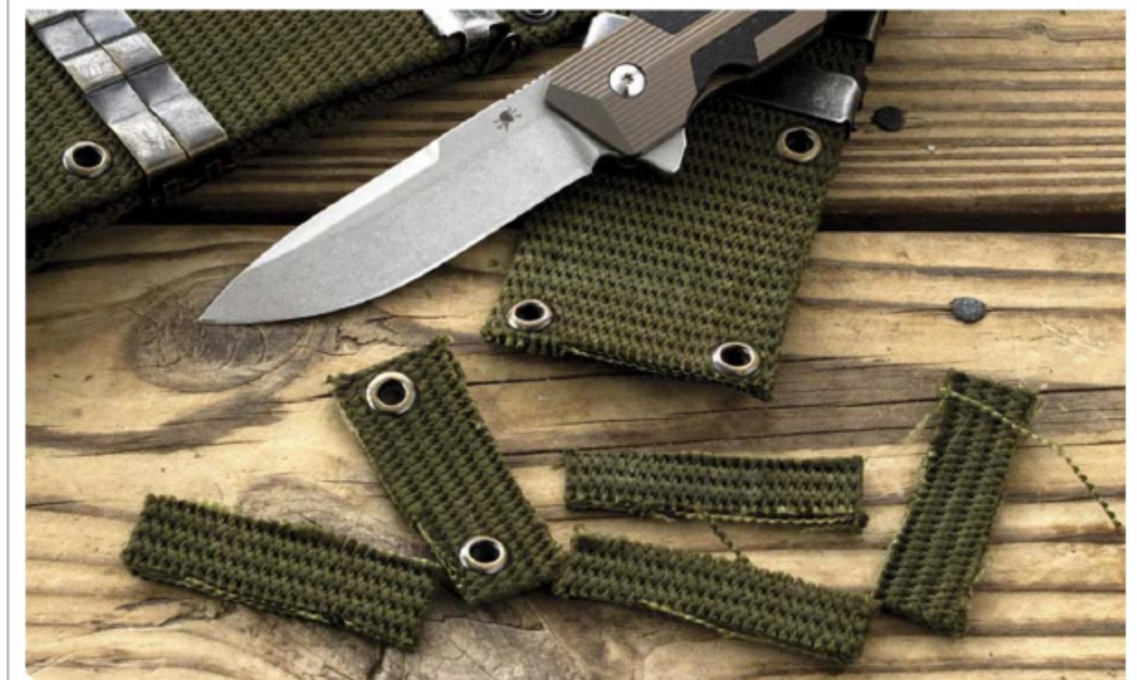
Bottom: I was able to get some very clean cuts on this military gun belt, made from very thick nylon webbing, without dulling the edge.
