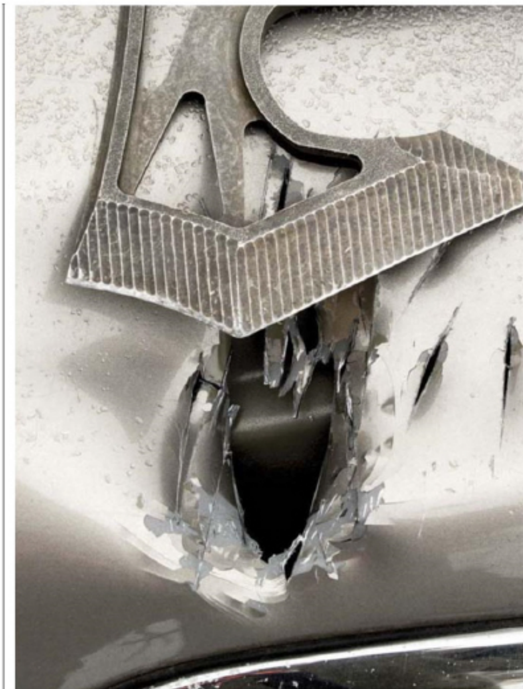
Utilizing the secondary point of the edge, I was able to open a large hole in the trunk lid like a can opener.
