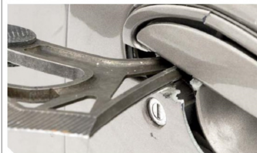
It was very easy to pop the lock out of the door with the spike.
