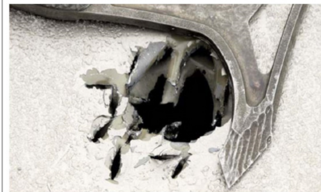
I was able to create a 2.5-inch-diameter hole in the trunk lid using the spike with very little effort.
