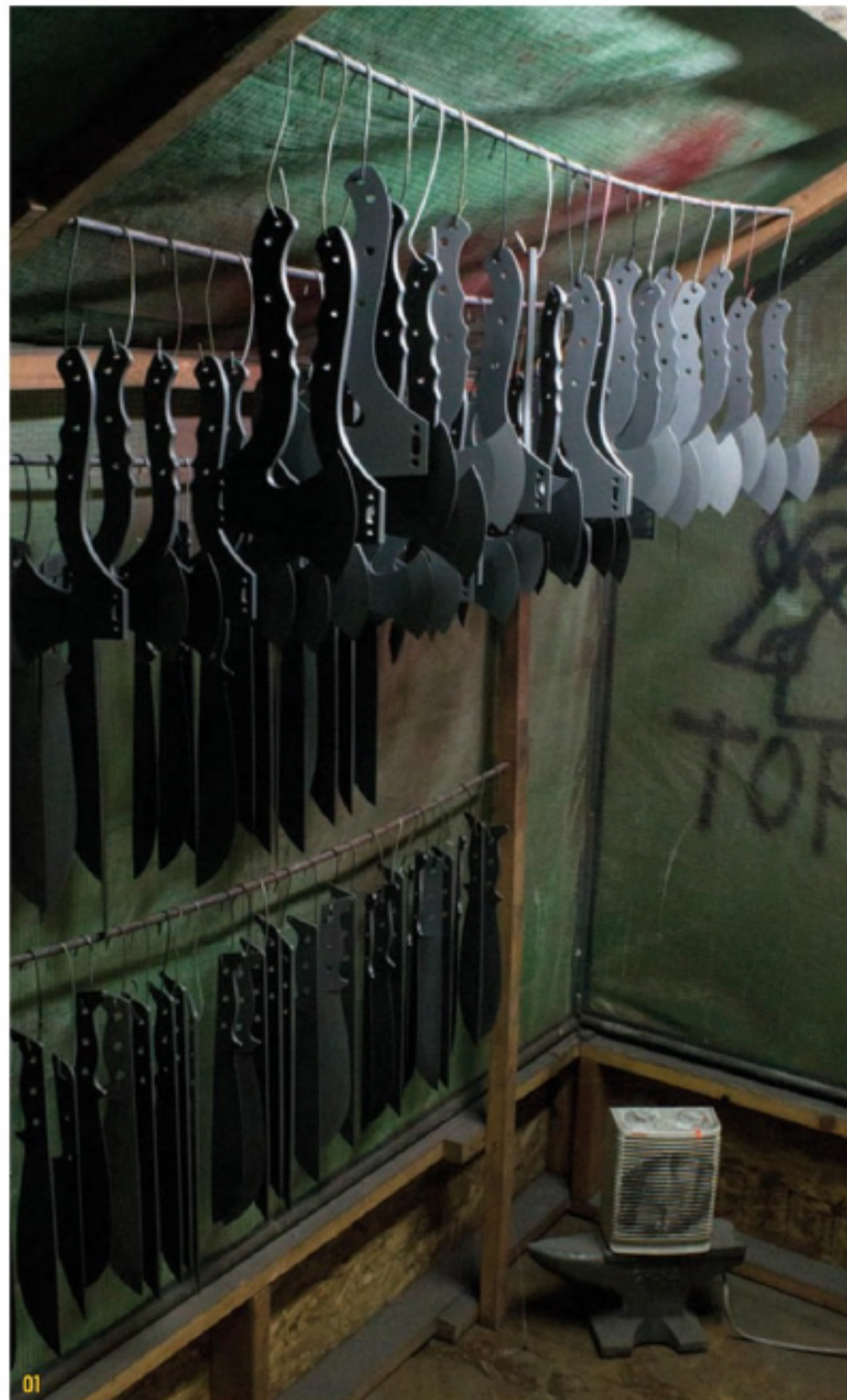
01: The "Greenhouse." Any knives that take clear Cerakote need to cure for about 5 days for the coating to fully harden—these coatings include tumbled, Black River wash, etc.
