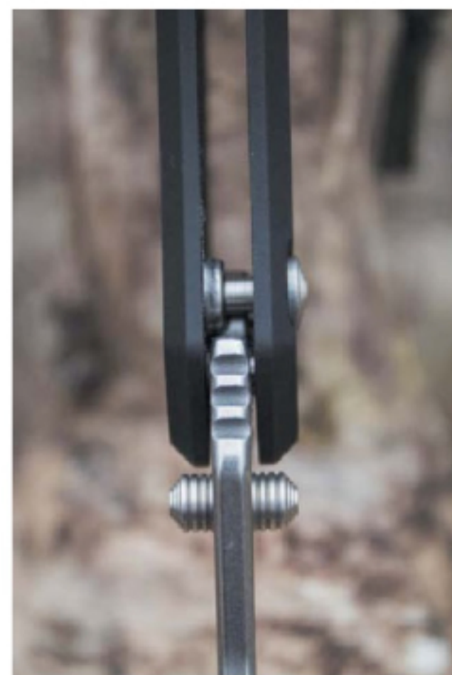
The button lock fits snugly into the groove, keeping the blade tight during use.
