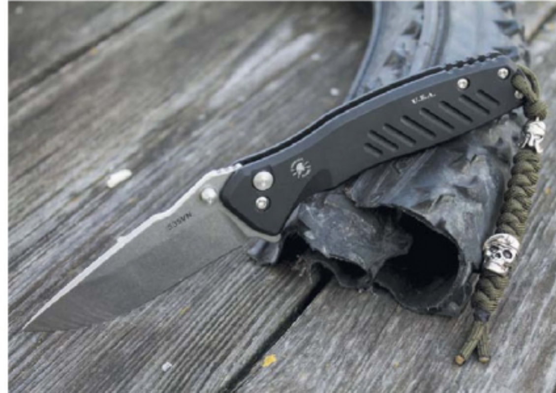
The author tested the Pallas on a bike tire and was able to slice right through it with a little bit of work. (He used wire cutters to cut the steel beads around the rim of the tire. Don't attempt to cut these with your knife; you will ruin it and most likely void any kind of warranty).
